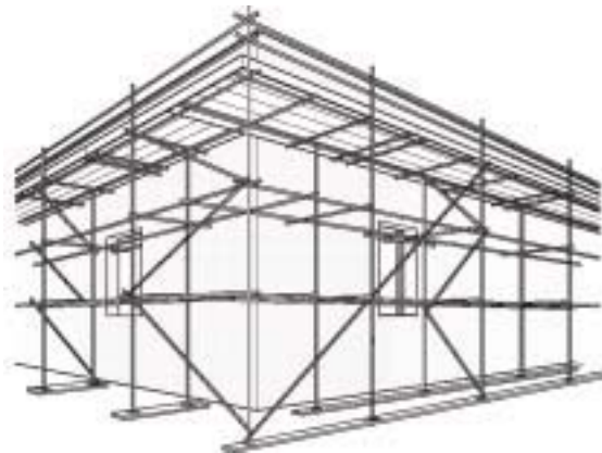
Typical independent tied scaffolding.
